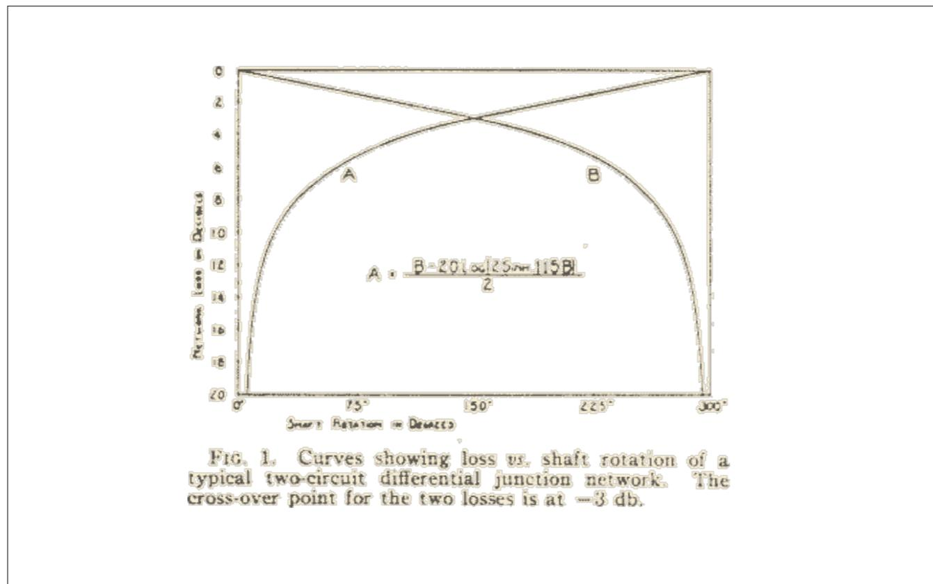
FIG. 1. Curves showing loss vs. shaft rotation of a typical two-circuit differential junction network. The cross-over point for the two losses is at -3 db.
