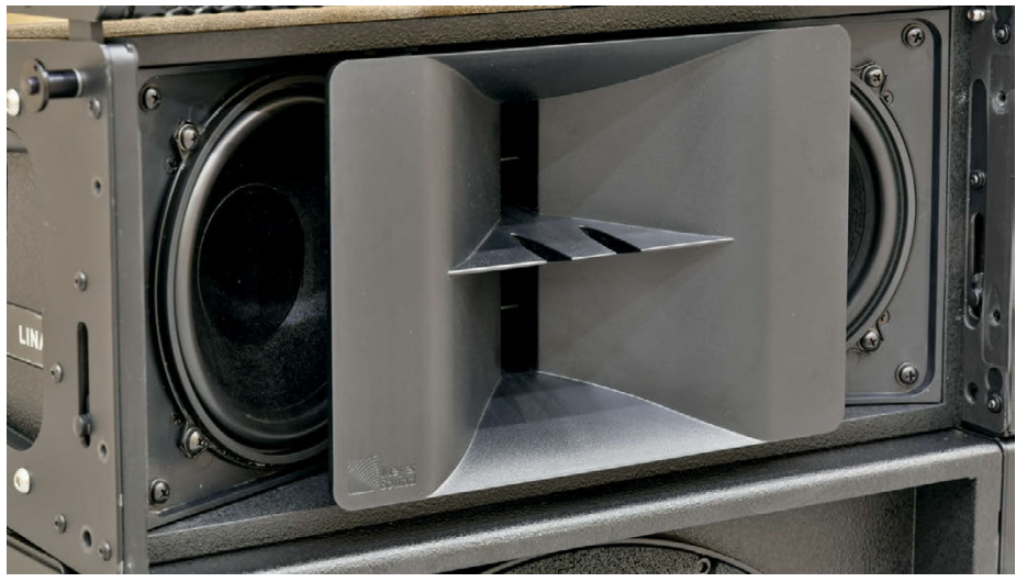
The LINA's HF The two 6.5" woofers can be identified behind the waveguide's sides
