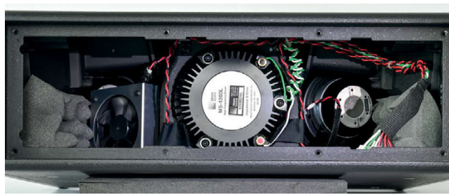
The LINA's two 6.5” woofers with neodymium drive , the HF driver with 3” cone in the middle, the left woofer is covered by a fan, which provides air movement in the cabinet if necessary
