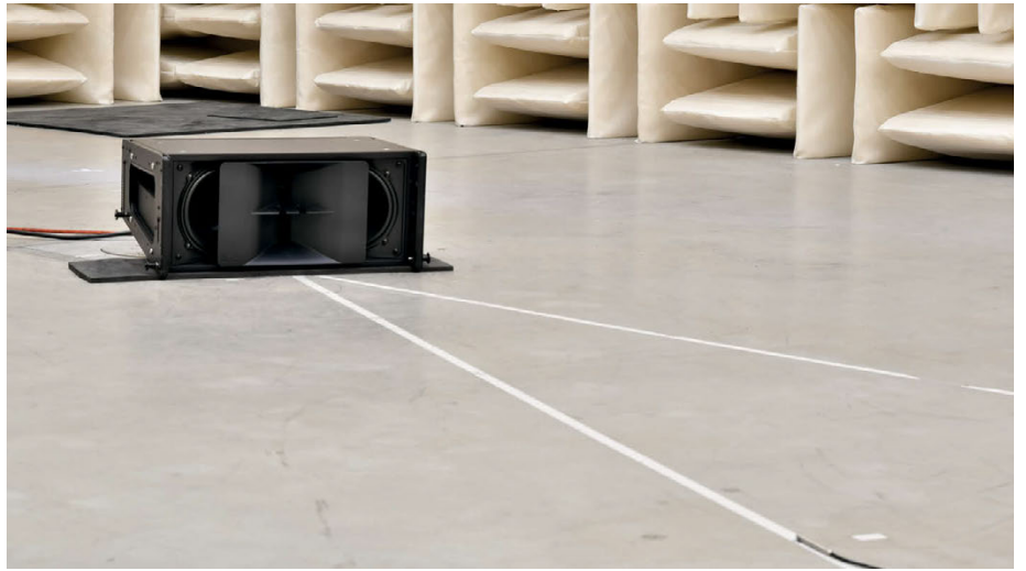
A single LINA prepared for a first measurement in an anechoic chamber (the microphone is located in the lower right corner)
