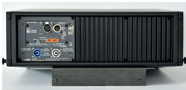
The LINA's rear with cooling profile and connection panel (the protective cover was temporarily removed for the photo)
