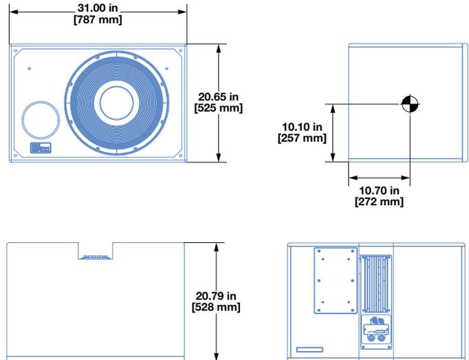
Part of Meyer Sound's cinema series, the X-400C Compact Cinema Subwoofer boosts low-frequency headroom in cinema applications and other fixed installations. The linear, self-powered X-400C offers similar sonic characteristics to the X-800C subwoofer—low-frequencies down to 20 Hz, clean, punchy transients, and excellent phase coherence—in a more compact cabinet that can be installed singly or as multiple units.
