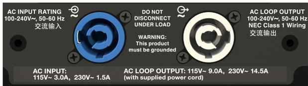
Figure 7: AC Input (Left) and AC Loop Output (Right) Connectors
