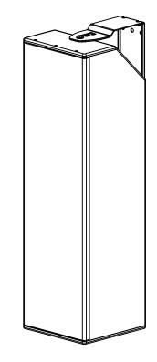
Figure 19: MUB-USW-210P Wall Mount, Vertical
