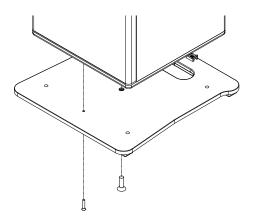
Figure 14: Base Plate Attachment to Loudspeaker, Exploded View
