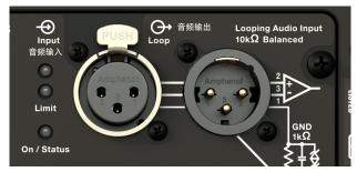
Figure 11: XLR 3-Pin Audio Connectors, Input and Loop Output
