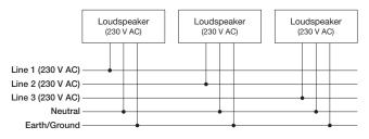
Figure 6: 230 V AC, 3-Phase Wye System (Single Line to Loudspeakers)
