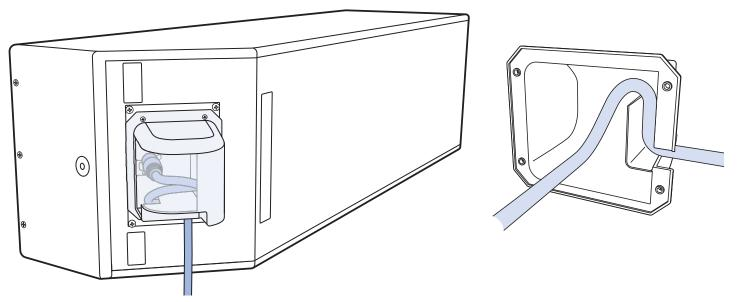
Figure 25: USW-210P with rigid rain hood (left) and interior cable routing illustration (right)
