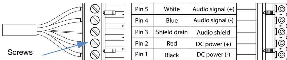
Figure 29: Pin Destinations for Phoenix 5-Pin Female Cable Mount Connector
