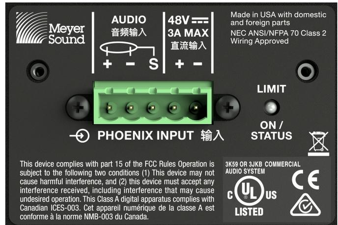
Figure 2: USW-112XP Rear Panel with Phoenix 5-pin Male Connector
