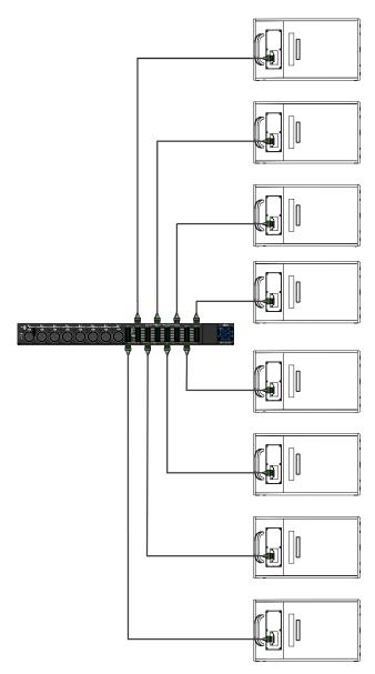
Figure 7: MPS-488HPp with Eight USW-112XP Loudspeakers
