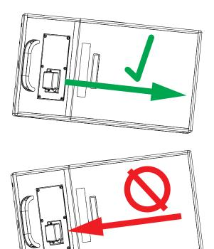
Figure 26: Horizontal Tilt-Away from Electronics Permissible (top); Horizontal Tilt-Toward Electronics **NOT** Permissible (bottom)
