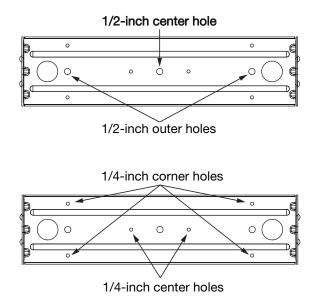
Figure 11: Mounting Hole Locations
