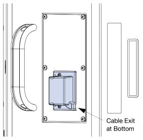
Figure 23: Only Permissible Horizontal Orientation
