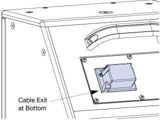
Figure 22: Only Permissible Vertical Orientation
