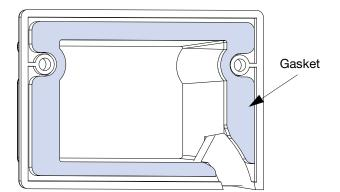
Figure 21: Rain Hood with Gasket Attached
