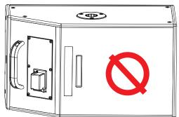
Figure 24: Downtilt Permissible (top); Uptilt **NOT** Permissible (bottom)
