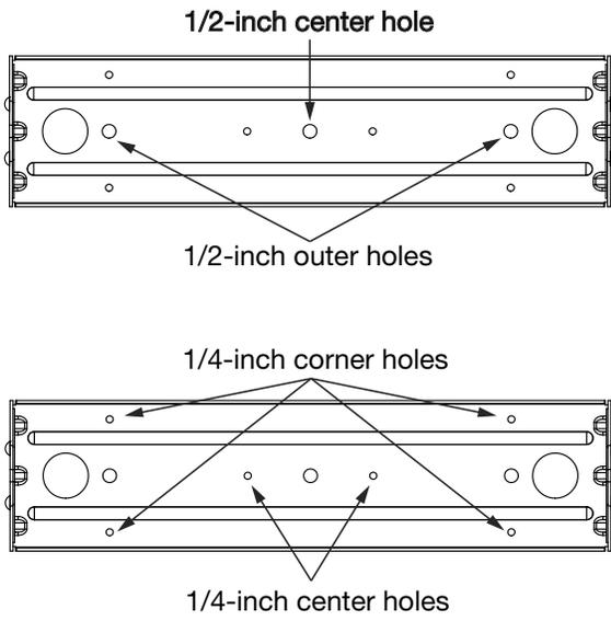
Figure 21: Mounting Hole Locations
