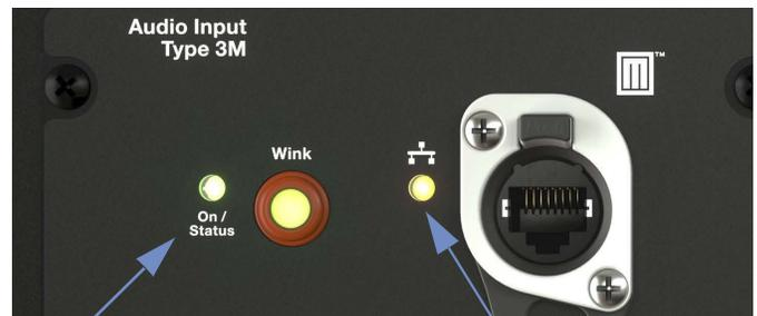
Figure 17: USW-112P On/Status LED and Ethernet connectivity LED
