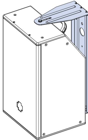
Figure 23: MUB-USW-112 Wall Mount, Vertical
