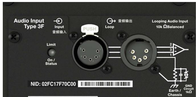
Figure 9: XLR 5-Pin Audio Connectors, Input and Loop Output
