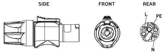
Figure 6: powerCON 20 Cable Mount Connector
