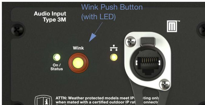
Figure 15: USW-112P Digital Audio Wink Push Button and LED
