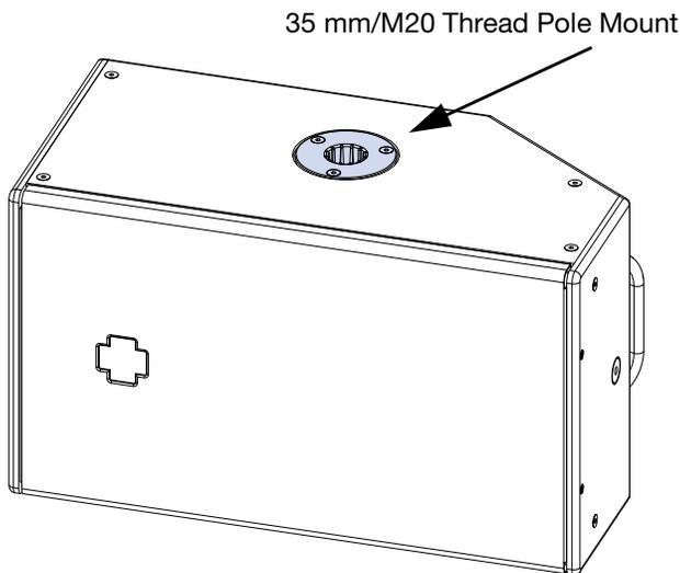
Figure 19: USW-112P Integral Pole Mount
