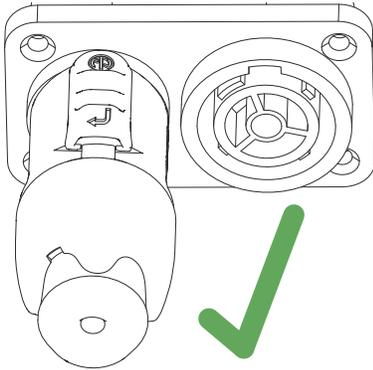
*Figure 8: Locked Connector Position*
