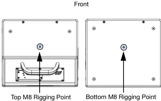
Figure 18: USW-112P Rigging Points
