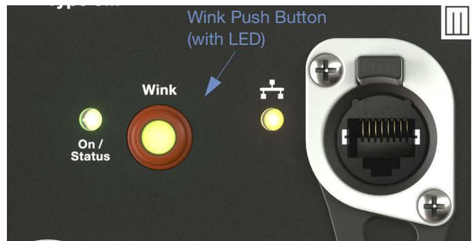
Figure 29: USW-112P Digital Audio Wink Push Button and LED
