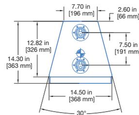
The UPA-2P loudspeaker provides high power output, low distortion, and consistent polar response in a compact, vented two-way enclosure. The loudspeaker features a 12 in cone low-frequency driver and a 3 in diaphragm compression driver coupled with a 45° symmetrical high-frequency horn. The versatile UPA-2P has a variety of sound reinforcement applications including as a main front-of-house loudspeaker in smaller venues (singly or in arrays) and as a delay or fill loudspeaker in larger systems.
