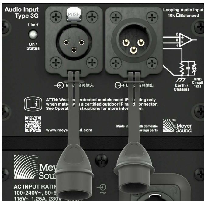
Figure 11: Weather-protected analog units have 3-pin XLR TOP audio connectors
