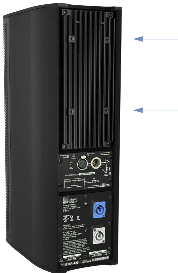
ULTRA-X20 Heat Sink Third-party Accessory Mounting Capability 5-inch x 2.75-inch (127 mm x 70 mm) Hole Pattern
