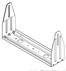
Width 23.14 in [494 mm] Height 4.50 in [114 mm]
