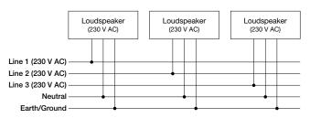
Figure 3: 230 V AC, 3-Phase Wye System (Single Line to Loudspeakers)
