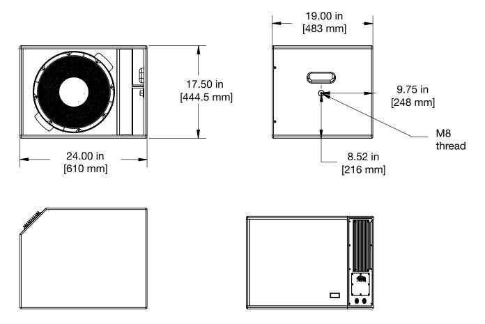
Figure 12: Ultra Reflex LF-15 Loudspeaker Dimensions
