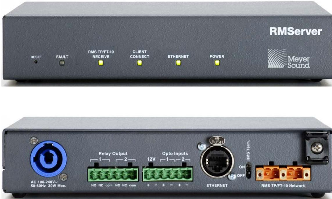
RMServer is a compact hardware unit that runs RMS over Ethernet. Situated between the computer running Compass and the loudspeaker cabinets, RMServer's two FT-10 ports can be connected to up to 50 RMS loudspeakers or 12 MPS-488HP power supplies. Since each MPS-488HP powers eight loudspeakers, one RMServer can monitor 96 48 V loudspeakers connected to MPS-488HPs that are equipped with the RMS option.
