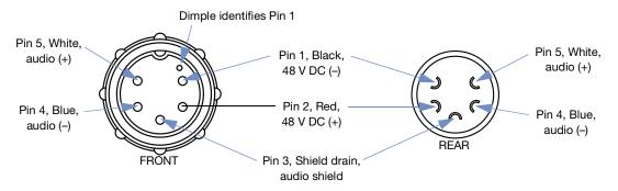
Pin Destinations for EN3 5-Pin Female Cable Mount Connector
