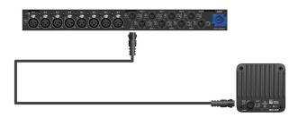
To join two cables, one with an EN3 5-pin male cable mount connector to one with an EN3 5-pin female cable mount connector, use an EN3 5-pin female-to-male cable coupler (PN 28.163.033.01).
