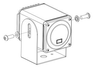
Secure the loudspeaker to the U-bracket using the two 3/8-inch-16 screws and two shoulder washers included with the MUB-MM-4XP. The shoulder washers should be placed between the screws and the outside of the U-bracket, with the shoulder oriented toward the loudspeaker. Do not yet tighten the U-bracket screws.
