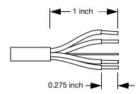
2. Insert the five exposed conductors into the five cable holes in a Phoenix 5-pin female cable mount connector. Use the following wiring scheme.
