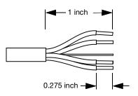
3. Solder the five exposed conductors to the five pins on the EN3 cord connector using the following wiring scheme.
