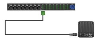
For an MPS-488HPE power supply, use an EN3 5-pin female to EN3 5-pin male cable.
