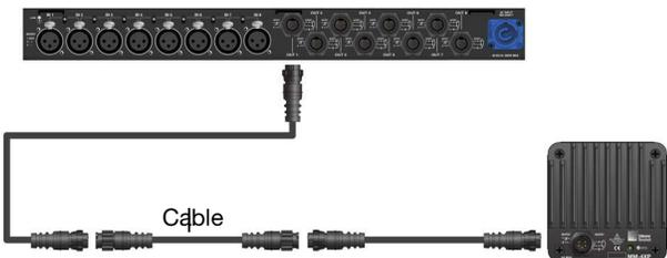
**CAUTION:** Make sure the MM-4XP loudspeaker cables are wired correctly. For details on assembling loudspeaker cables, see “Assembling Loudspeaker Cables” on page 17.
