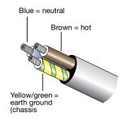
AC Cable Wiring Scheme
