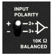
MM-10ACX Input Polarity Switch
