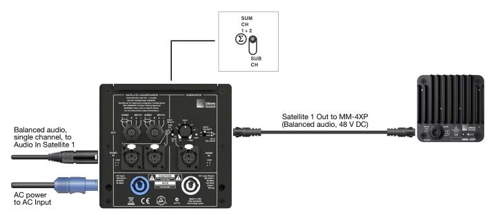
MM-10ACX Single-Channel Satellite System (Shown with EN3 Connectors)
