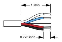
3. Solder the five exposed conductors to the five pins on the EN3 cord connector using the following wiring scheme.
