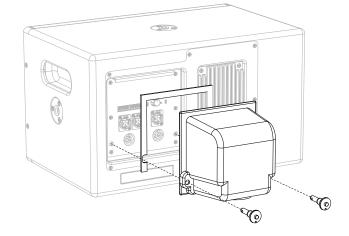
4. Secure the rain hood to the user panel by inserting the lock pins in the two bottom holes. Insert the pins all the way so they lock.
