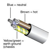
AC Cable Wiring Scheme
