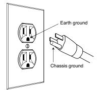
Do not use a ground-lifting adapter or cut the AC cable ground pin.
