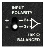
MM-10AC Input Polarity Switch
