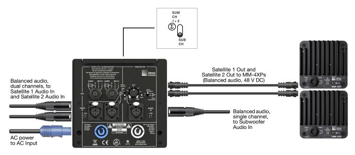
MM-10ACX Dual Channel + Sub Channel System (Shown with EN3 Connectors)
