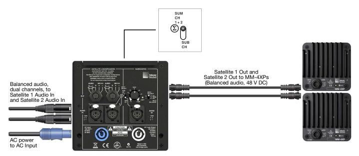
MM-10ACX Dual-Channel Satellite System (Shown with EN3 Connectors)
