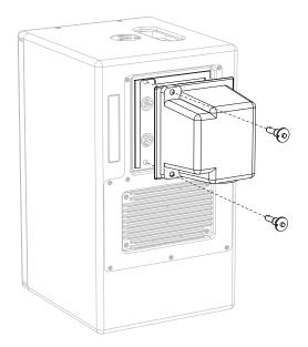
5. Secure the rain hood to the user panel by inserting the lock pins in the two left holes. Insert the pins all the way so they lock.
