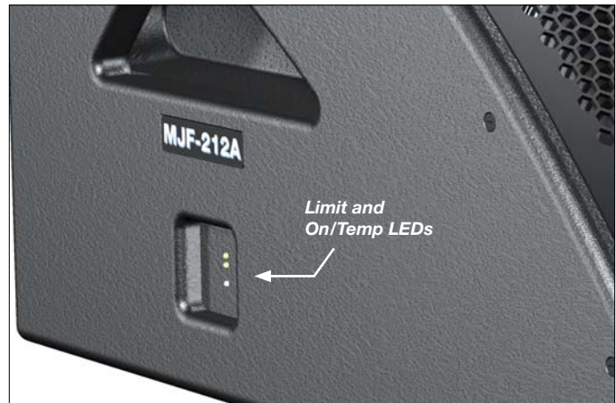
Figure 3.3: Limit LEDs on the side of the cabinet mirror the limiter activity of the user panel on the opposite side
