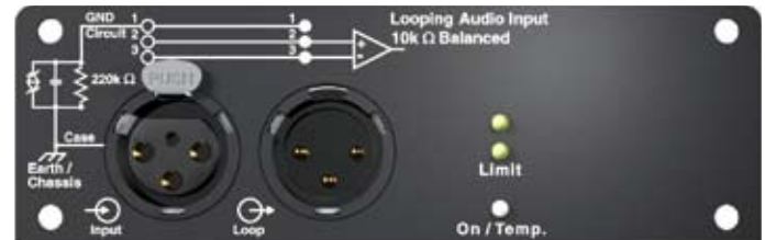
Figure 3.1. Side panel audio input connectors
