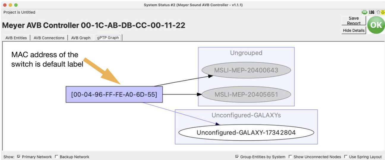
*GALAXY, Two Milan Endpoint Input Modules, and Network Switch—AVB Controller, gPTP Tab, Display of gPTP Network Paths*
