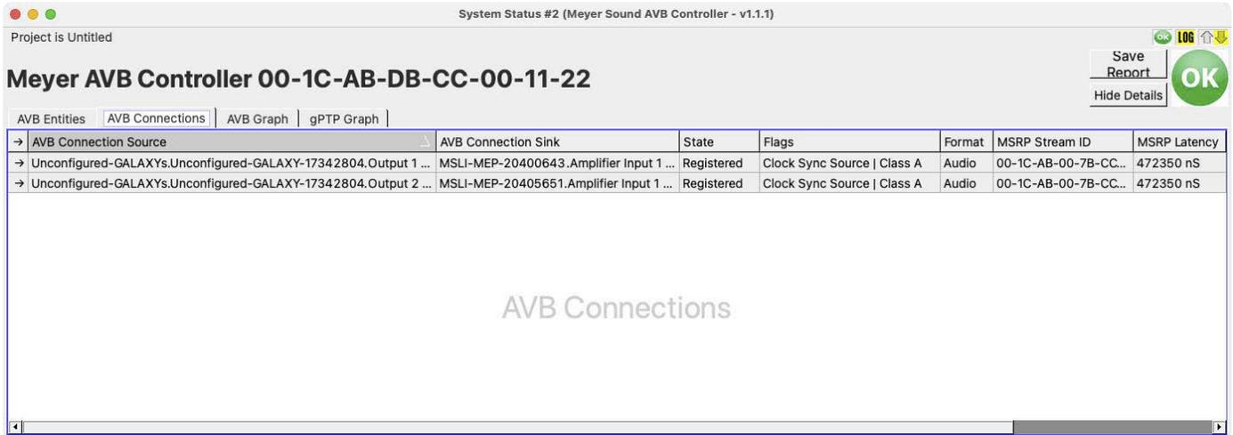
AVB Controller, AVB Connections Tab, Each AVB Connection and Details are Listed
