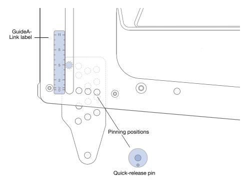
Figure 9: LINA Rear GuideALink Label and Pinning Positions
