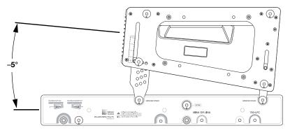
Figure 37: MG-MINA Grid with Groundstacked LINA, -5 Degrees Downtilt
