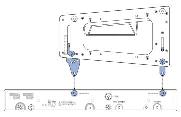
Figure 35: MG-MINA Grid with Groundstacked LINA, 0 Degrees
