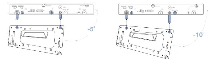
Figure 21: MG-MINA/LINA/750-LFC Grid, Maximum Uptilt Orientation, -5 and -10 Degrees
