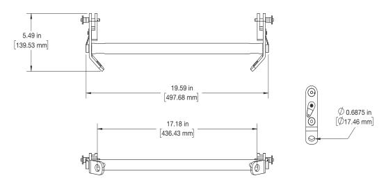
Figure 29: PBF-LINA Pull-Back Frame Dimensions
