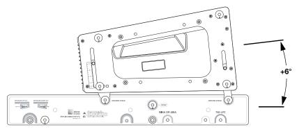
Figure 36: MG-MINA Grid with Groundstacked LINA, +6 Degrees Uptilt
