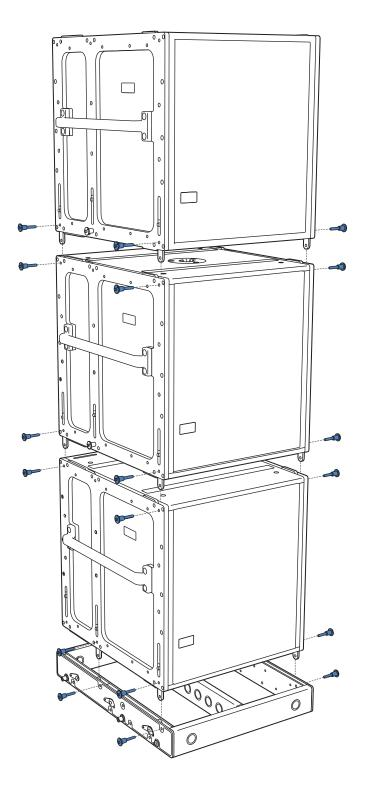
Figure 39: MG-MINA/LINA/750-LFC Grid with Groundstacked 750-LFCs, Exploded View
