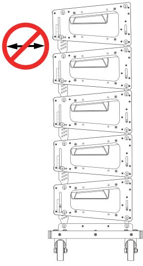
Figure 63: Proper/Improper Stack Movement Direction
