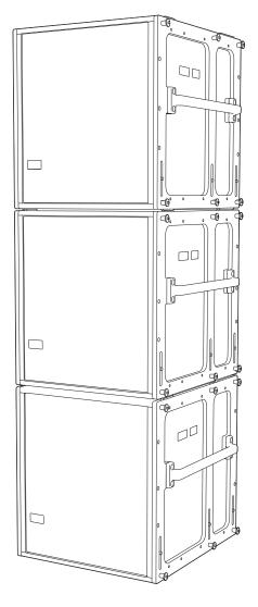
Figure 4: 750-LFC Groundstack (With Rigging)
