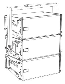
Figure 42: MYA-MINA/LINA Mounting Yoke with MPA-3 bracket and Three LINA Loudspeakers
