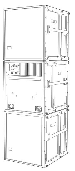
Figure 5: 750-LFC Cardioid Groundstack (Without Rigging)
