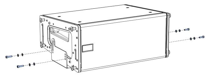
Figure 54: Floor-Mounted MUB-MINA/LINA with One LINA
