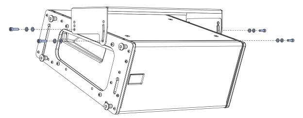
Figure 56: Ceiling-Mounted MUB-MINA/LINA with One LINA
