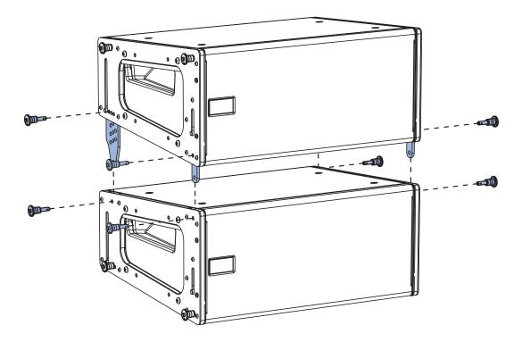
Figure 6: LINA GuideALinks with Quick-Release Pins
