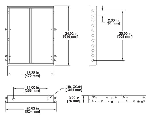
Figure 17: MG-MINA/LINA/750 Grid Dimensions
