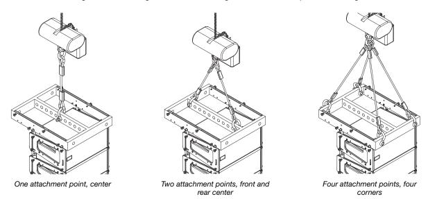
Figure 23: Examples of Pickup Configurations with One Motor
