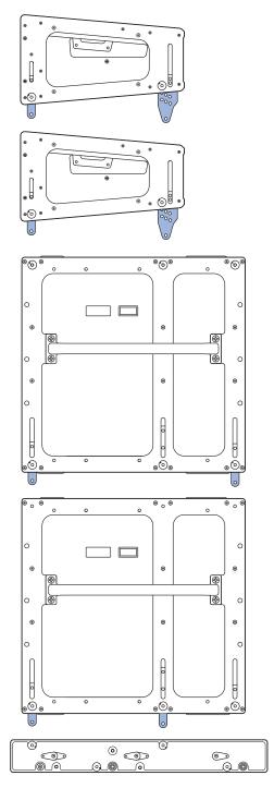
Figure 14: Groundstacked LINA and 750-LFC with GuideALink Attachments
