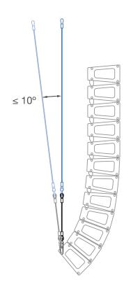
Figure 31: Limit on Pull-back Chain Deviation from 0 degrees vertical
