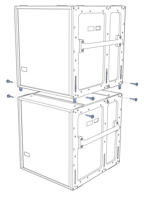
Figure 11: 750-LFCs with MRK-750 Rigging Kit, GuideALinks and Quick-Release Pins
