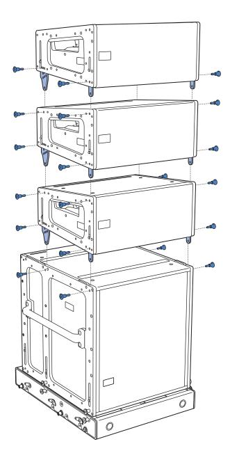
Figure 40: LINAs Groundstacked on 750-LFC, Exploded View
