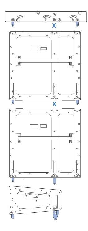
Figure 13: FlownMG-MINA/LINA/750-LFC, 750-LFC and LINA with GuideALink Attachments
