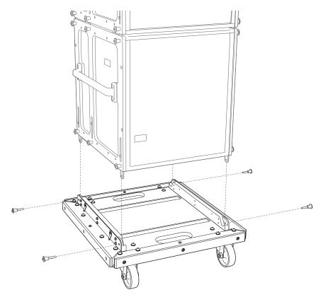
Figure 65: MCF-750 Caster Frame with 750-LFC Stack, Exploded View
