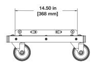
Figure 60: MCF-MINA/LINA Caster Frame Dimensions
