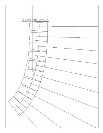
Figure 24: MAPP Showing LINA Array with Center of Gravity
