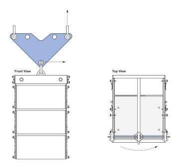
Figure 27: MVP Motor Vee Plate, Pulling Up on Either Motor Rotates the Grid
