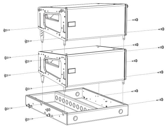
Figure 34: MG-MIN/LINA/750-LFC Grid with Groundstacked LINA
