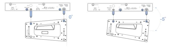
Figure 20: MG-MINA/LINA/750-LFC Grid, Maximum Downtilt Orientation, 0 and -5 Degrees
