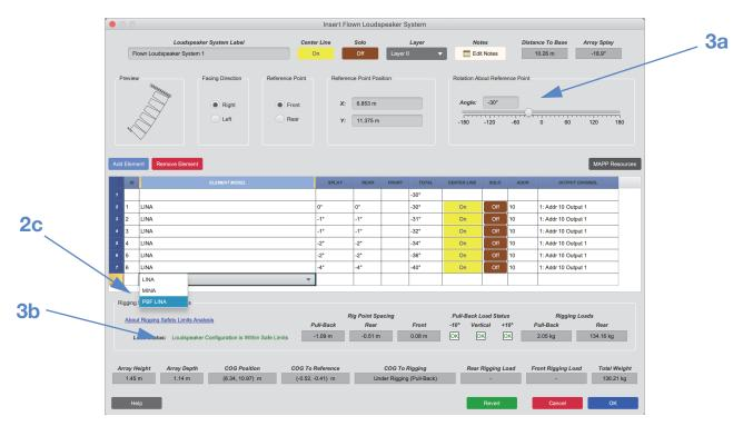
Figure 33: MAPP Display Window Shows Addition of Pull-Back Frame Brings Loudspeaker Configuration to Within Safe Limits
