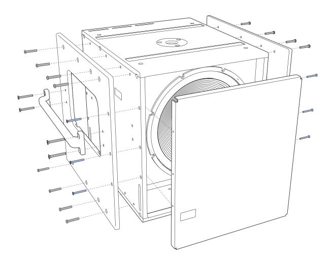
Figure 1: Removing Existing End Frames and Grille
