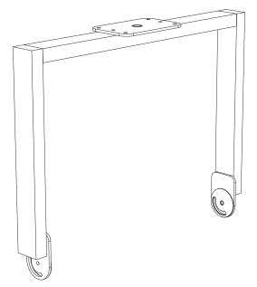
Figure 41: MYA-MINA/LINA Mounting Yoke
