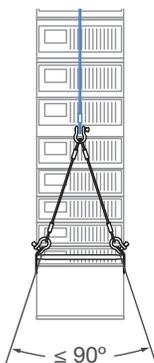
Figure 30: Bridle Apex Angle Limitation for PBF-LINA Pull-back Frame
