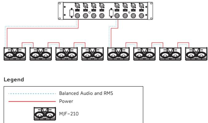
MDM-832 Connected to MJF-210 Loudspeakers with Separate Cables and Loop Outputs
