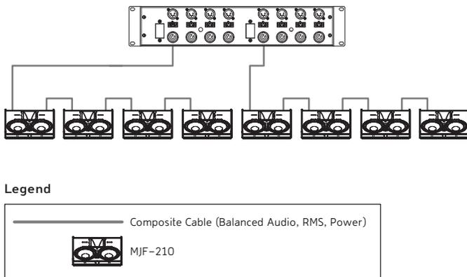
MDM-832 Connected to Loudspeakers with Composite Cables and Loop Outputs
