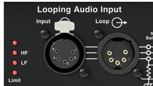
Figure 13: XLR 5-Pin Audio Connectors, Input and Loop Output
