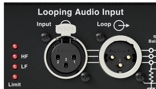
Figure 14: XLR 3-Pin Audio Connectors, Input and Loop Output
