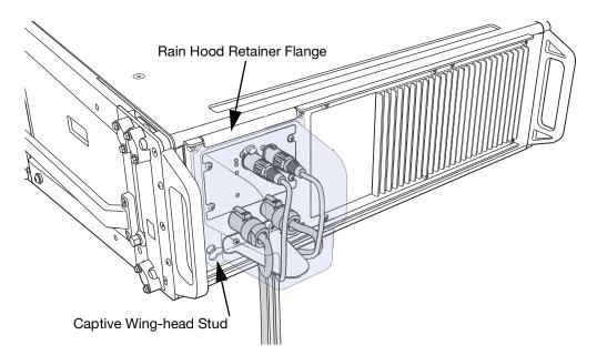
Figure 28: Routing Signal and Power Cables Through Rain Hood and Around Baffle
