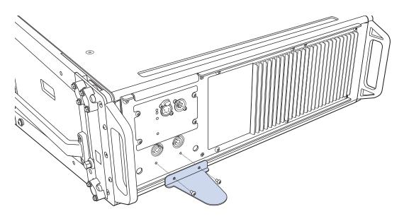
Figure 27: Attaching Rain Hood Baffle to LEOPARD Loudspeaker User Panel
