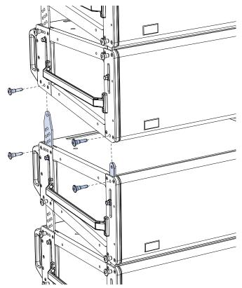
Figure 16: LEOPARD GuideALinks with Quick-Release Pins, Exploded View
