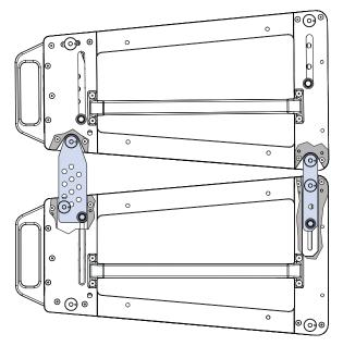
Figure 17: LEOPARD GuideALinks (Exposed) Attached at 0.5 Degrees
