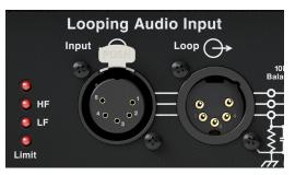
Figure 13: XLR 5-Pin Audio Connectors, Input and Loop Output
