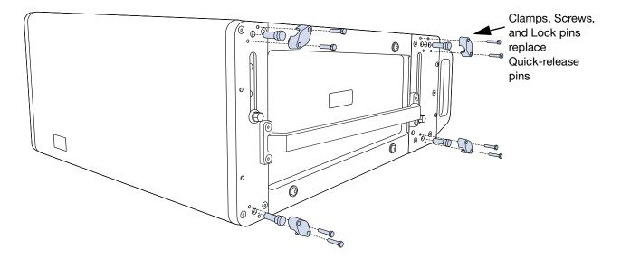
Figure 26: Ultra Weather Protection LEOPARD Loudspeaker Version has Clamps, Screws, and Lock pins that replace standard version quick-release pins
