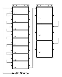
Figure 4: Flown Separate Arrays
