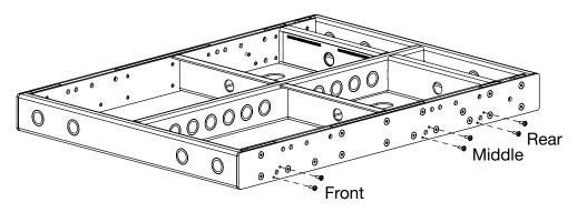
Figure 25: Blanking Screws (6 per side) to Prevent Corrosion at Unused Pin Locations for Ultra Weather Protection Grid
