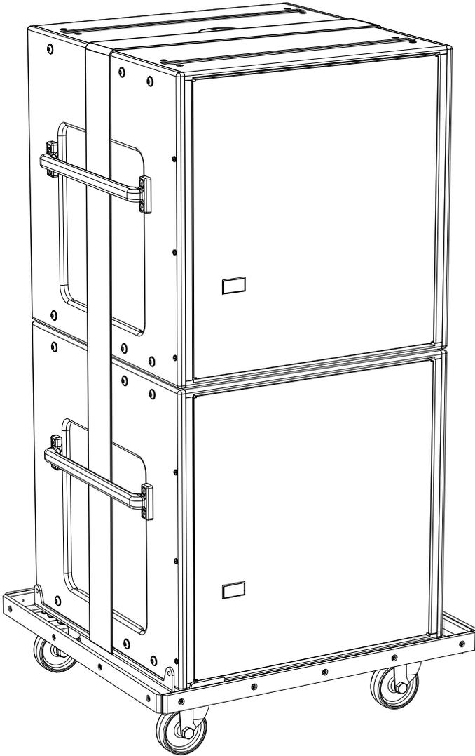
*MCF-900-LFC Caster Frame, (2) 900-LFCs (without Rigging), and Straps (Not Included)*
