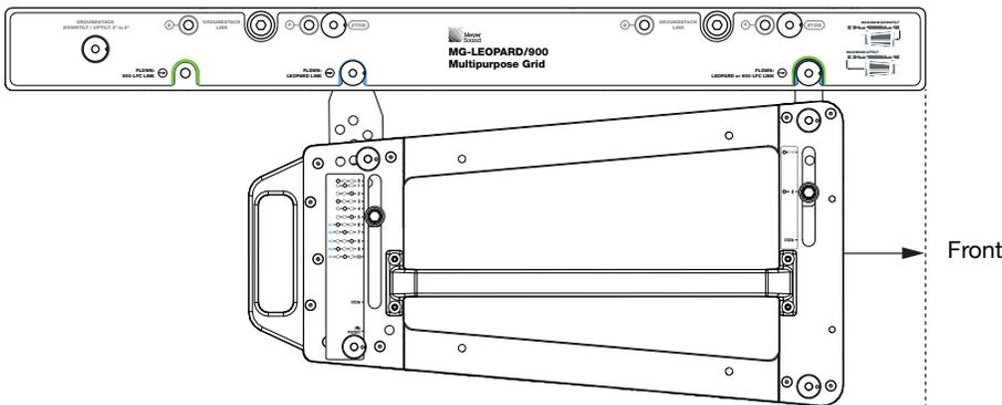
*MG-LEOPARD/900-LFC Grid Oriented for Maximum Array Downtilt (Forward)*
