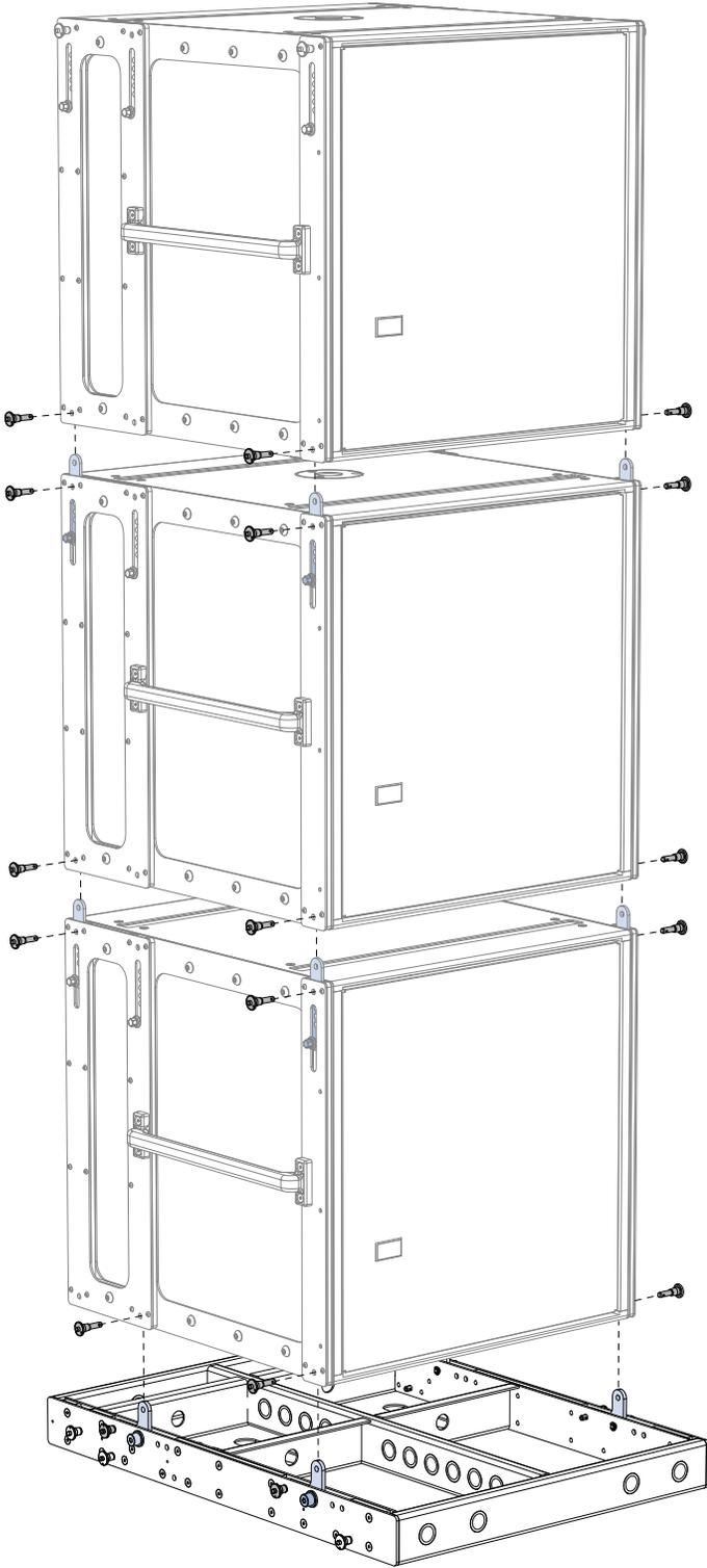
MG-LEOPARD/900-LFC Grid with Groundstacked 900-LFCs, Exploded View
