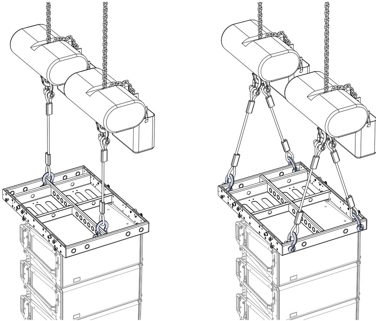
*2 Motors – 2 Pickup Points, Front and Rear (Left); 2 Motors – 2 Pickup Points, Front and Rear Side Bridles (Right)*
