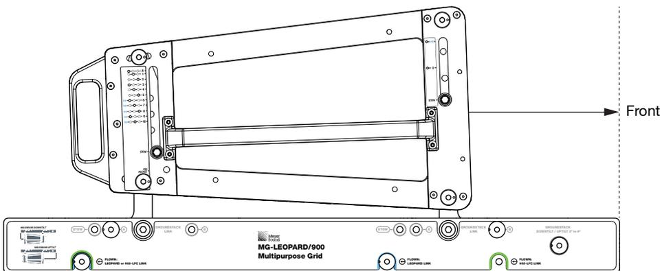
MG-LEOPARD/900-LFC Grid Oriented for Groundstack with Down-tilt (Rearward)
