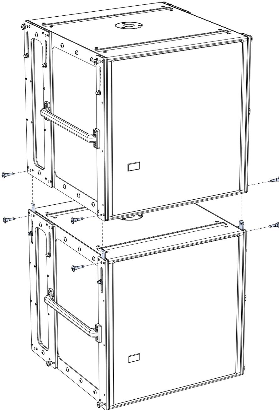
*900-LFCs with MRK-900-LFC Rigging Kit, GuideALinks and Quick-Release Pins, Exploded View*
