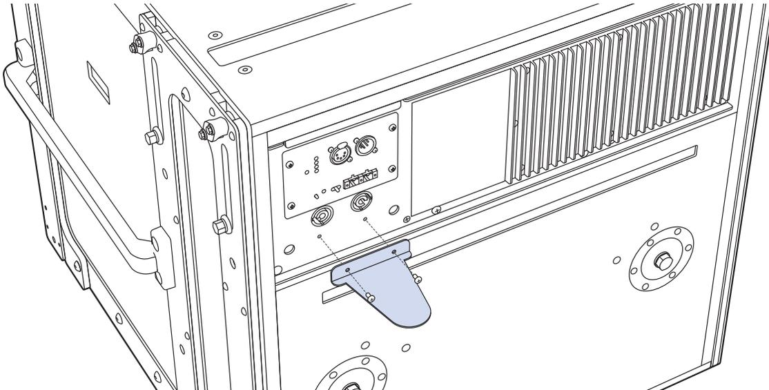
*Attaching Rain Hood Baffle to LEOPARD Loudspeaker User Panel*
