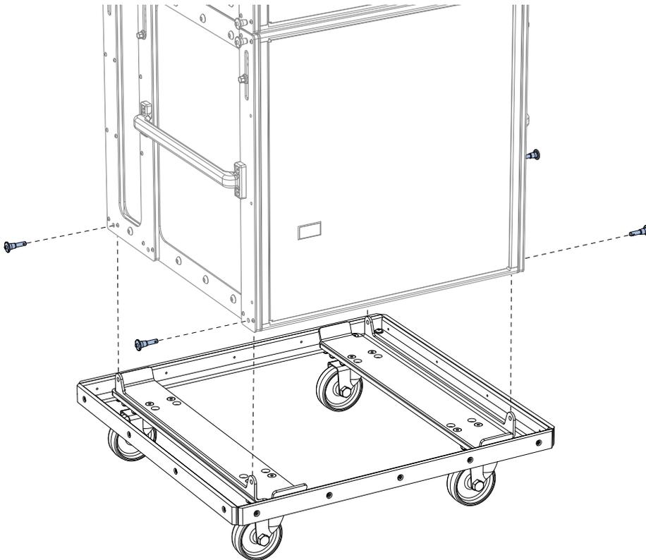
*MCF-900-LFC Caster Frame with 900-LFC Stack, Exploded View*
