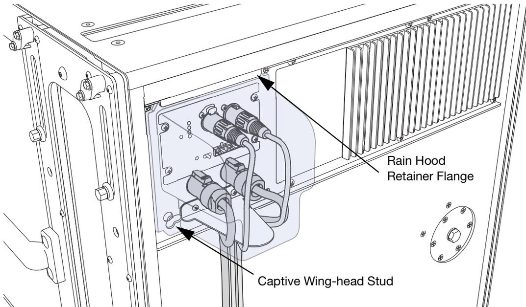
*Routing Signal and Power Cables Through Rain Hood and Around Baffle*
