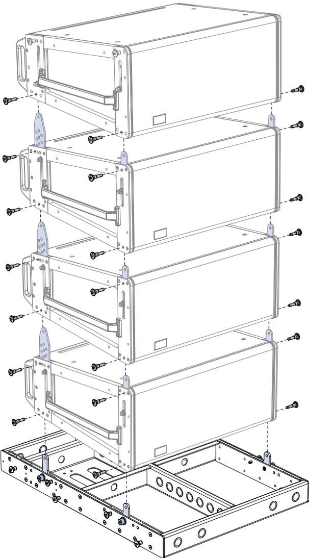
*MG-LEOPARD/900-LFC Grid with Groundstacked LEOPARDS, Exploded View*
