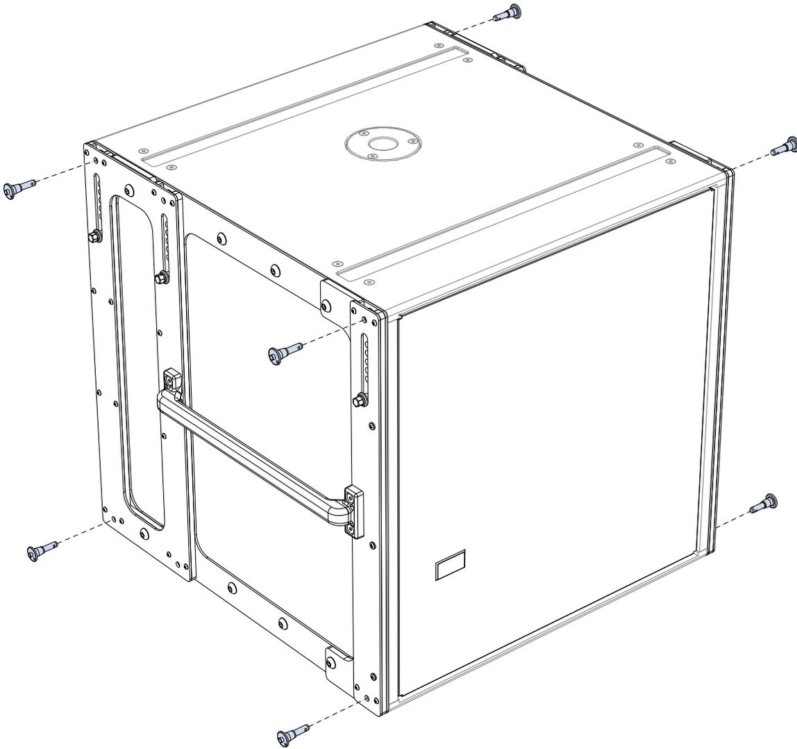
*Inserting Quick-Release Pins into 900-LFC Loudspeaker Rigging*
