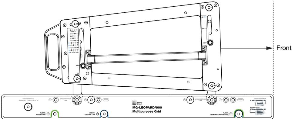
MG-LEOPARD/900-LFC Grid Oriented for Groundstack with Uptilt (Forward)
