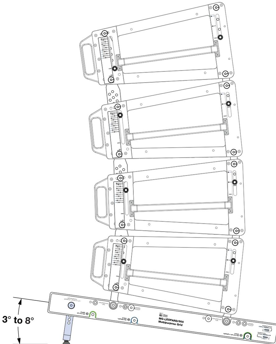
*MG-LEOPARD/900-LFC Grid with Optional Angle Feet, 8 Degrees of Downtilt*
