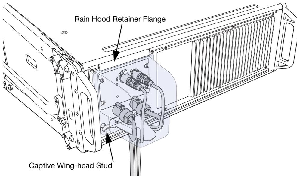
*Routing Signal and Power Cables Through Rain Hood and Around Baffle*
