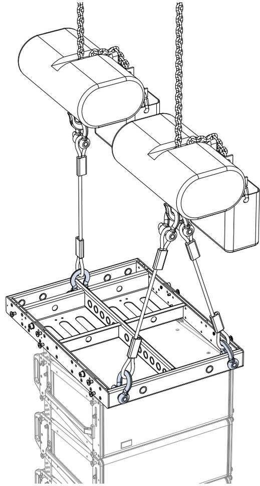
2 Motors – 3 Pickup Points, Rear Bridle (Left); 2 Motors – 3 Pickup Points, Front Bridle (Right)
