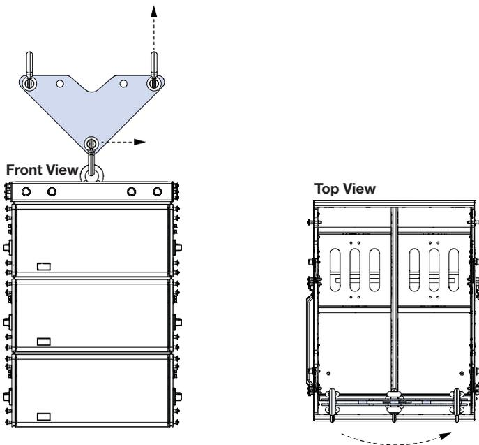
*MVP Motor Vee Plate, Pulling Up on Either Motor Rotates the Grid*
