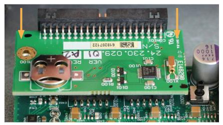
12. Fasten the provided PCB to the main PCB using the provided screw, applying 5–6 in-lbs (0.56–0.68 N·m) of torque.
