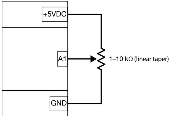
*External Potentiometer connected to ADC Input A1, Ground, and 5 V DC*
