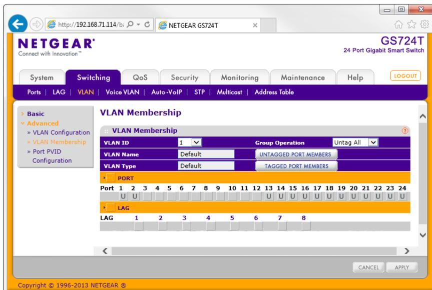
**NOTE:** The default VLAN maintenance port is 1. This must be U (untagged) on VLAN ID 1.
