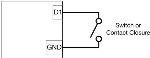
External Switch of Contact Closure connected to Logic Input D1
