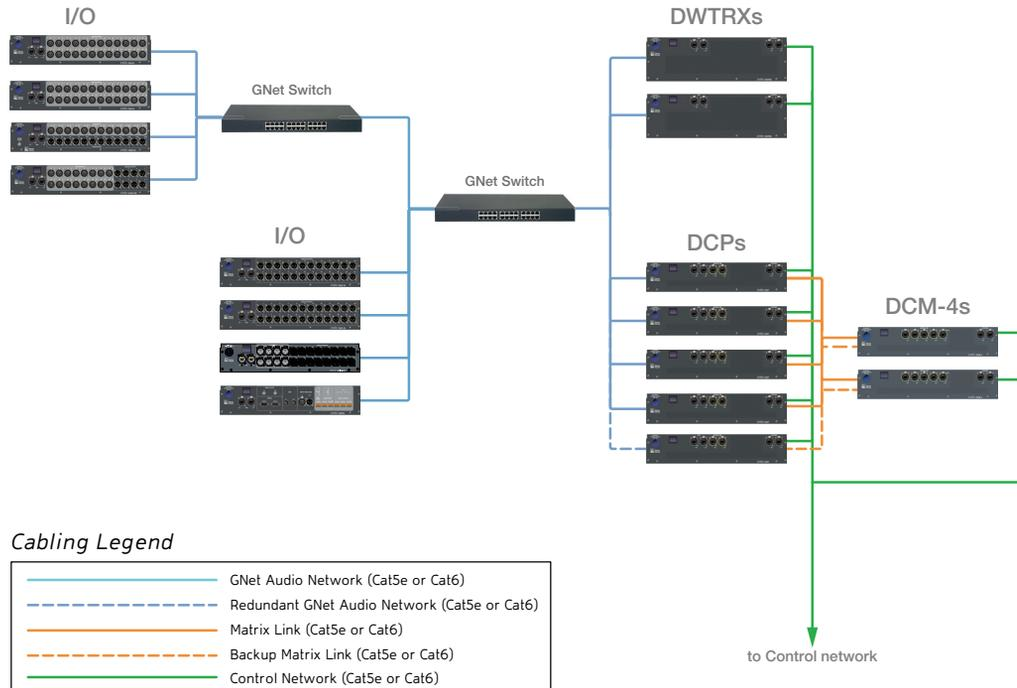
This distributed system features two racks of I/O modules in different locations, connected to an additional switch. DAI, DAO, DAIO-816, and DAIO-168 modules provide 68 analog inputs and 72 analog outputs. A DDIO module provides 24 digital inputs and 24 digital outputs. One DGPIO provides MIDI, serial, and Phoenix connections. Two DWTRX modules allow the playback of up to 500 channels on 144 busses, and recording of up to 144 channels.
