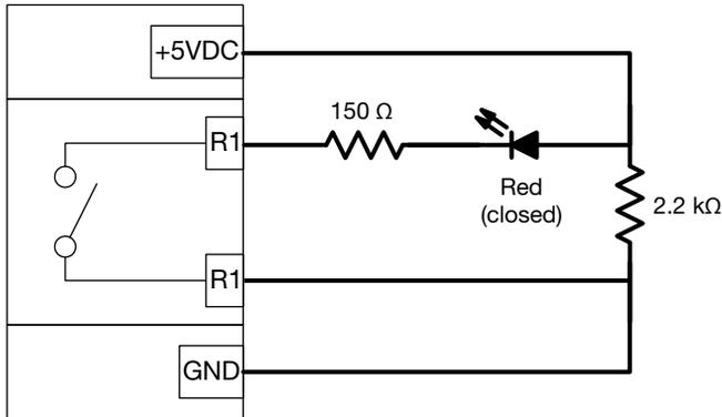
*External LEDs connected to Relay Output R1*
