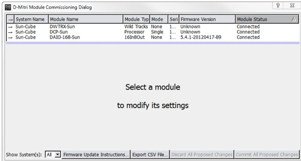
5. To filter the display of D-Mitri modules based on their system, select a system from the Show System menu at the bottom of the window.
