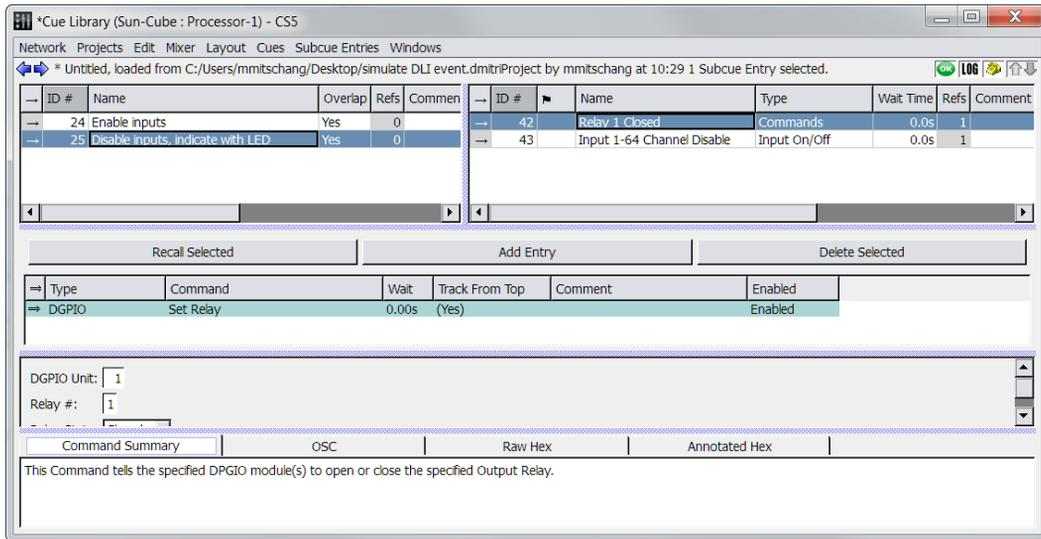
*Cue for Enabling Inputs and Closing a Relay*
