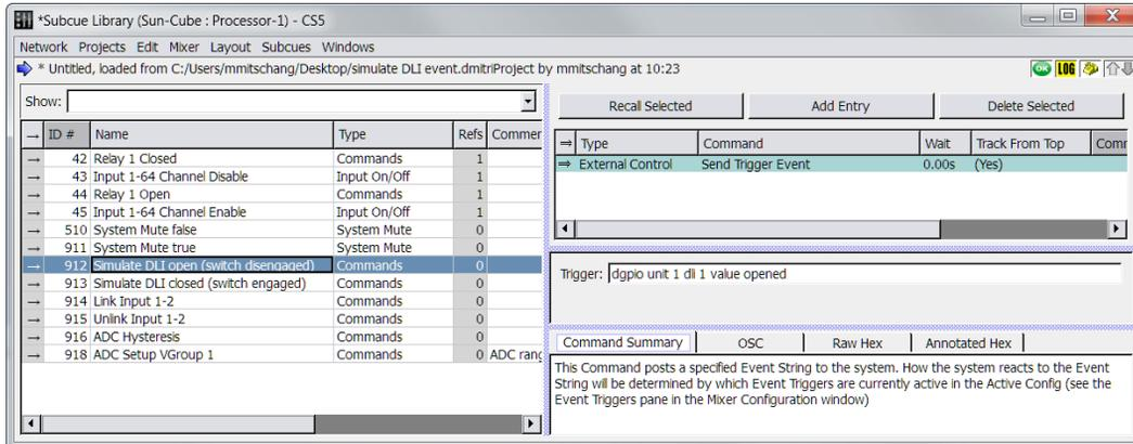
*Testing an Event Trigger with a Send Trigger Event command subcue*
