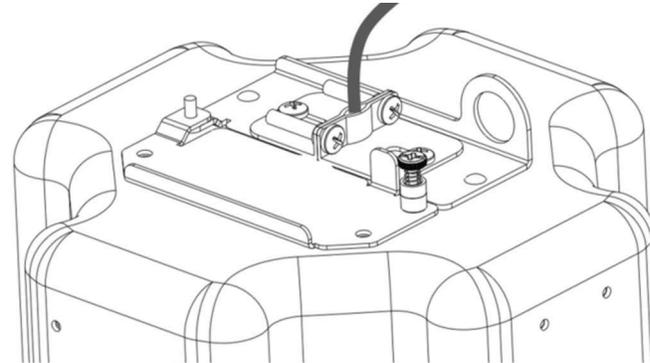
Figure 12: Clamping the wire
