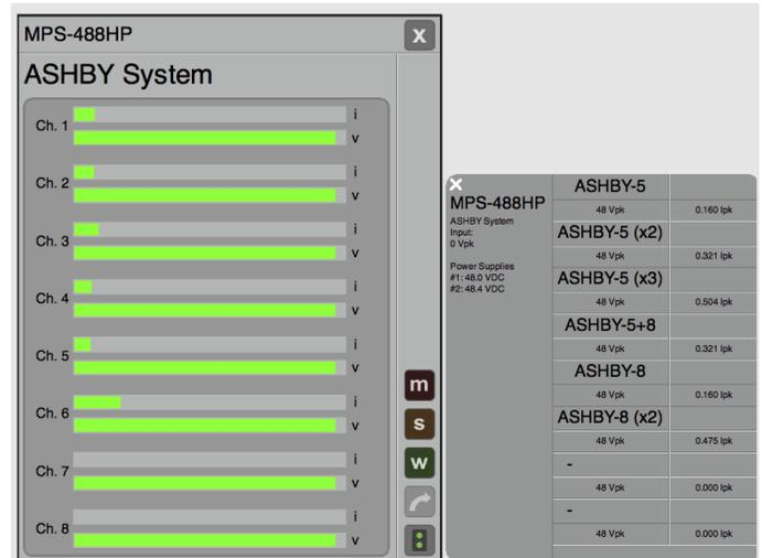
Figure 6: Voltage and current draw for connected loudspeakers in Compass
