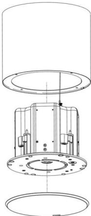
Figure 23: Installing an Ashby loudspeaker into a Meyer Sound pendant
