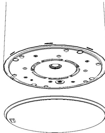
Figure 24: Fitting the grille frame onto an Ashby loudspeaker in a pendant
