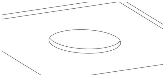
Figure 14: Cutting a hole in the ceiling with template provided
