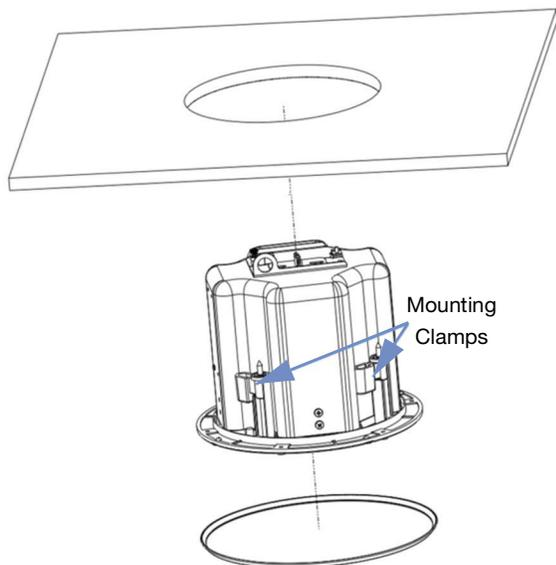
Figure 15: Inserting the loudspeaker into the ceiling
