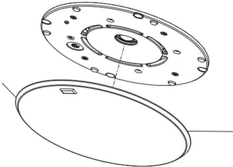
Figure 18: Placing the loudspeaker grille on the loudspeaker
