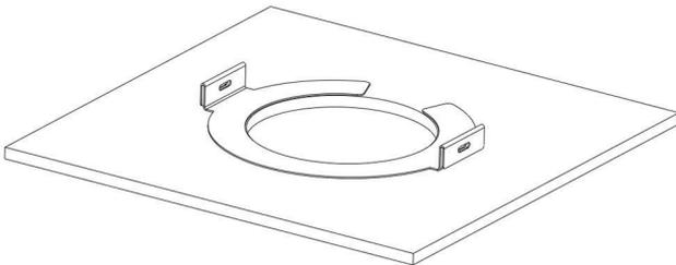
Figure 7: Using a C-ring to reinforce a brittle ceiling
