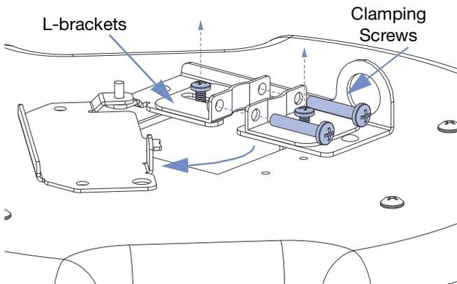
Figure 11: Removing clamping screws
