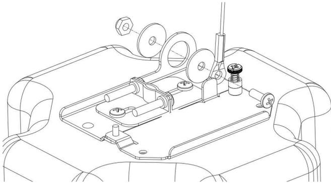
Figure 22: Attaching a safety lanyard
