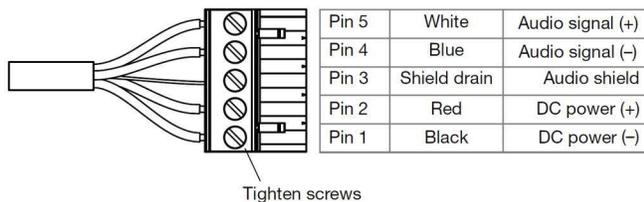
Figure 3: Belden 1502 multiconductor cable
