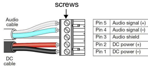
Figure 4: Separate Cables for DC Power and Balanced Audio
