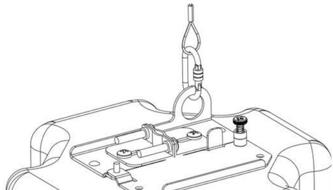
Figure 21: Attaching a safety lanyard for secondary support
