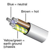
AC Cable Wiring Scheme
