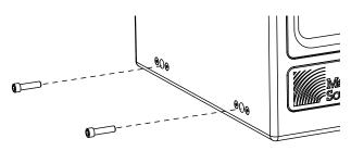
2. Secure the left bracket to the left side of the loudspeaker with two of the removed screws and two of the included flat washers.
