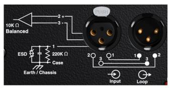
Acheron Audio Connectors, Input and Loop Output
