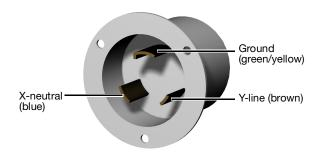
The Acheron requires a grounded outlet. To operate safely and effectively, it is extremely important that the entire system be properly grounded.
