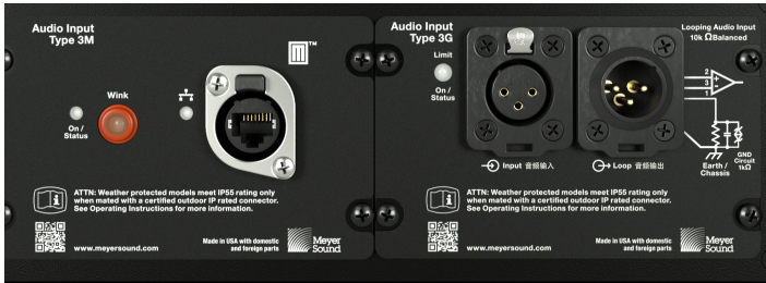
Figure 10. 2100-LFC User Panel, Audio Inputs, Sealing Caps Not Depicted
