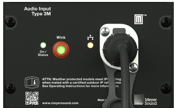
Figure 12. On/Status LED, Wink Button/LED, Network Connectivity LED, and Network Connector.
